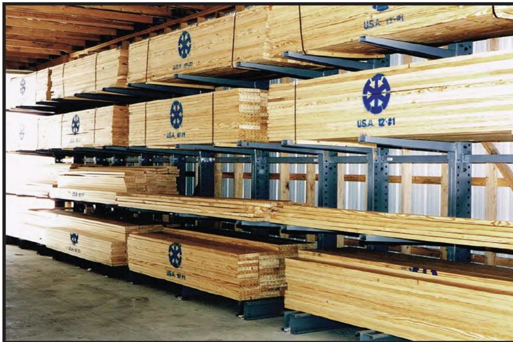
MECO OMAHA cantilever rack application consisting of uprights, arms and braces.
